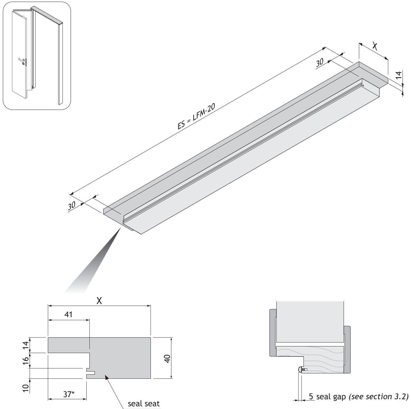
The dimension marked with (\*) vary according to the seal gap dimensions.
