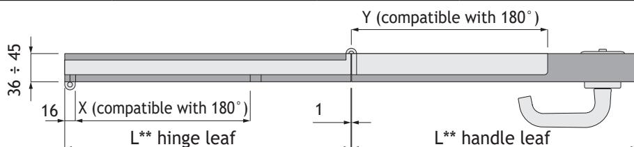
(\*\*) Hinge leaf and handle leaf widths are calculated with a reciprocal distance of 1 mm.
