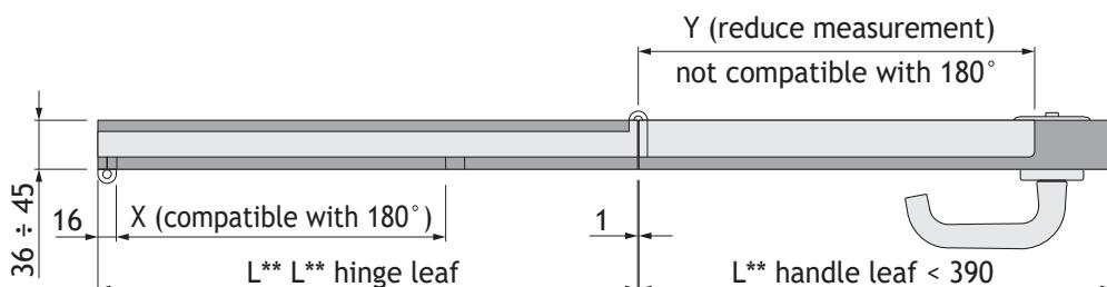
(\*\*) Hinge leaf and handle leaf widths are calculated with a reciprocal distance of 1 mm.
