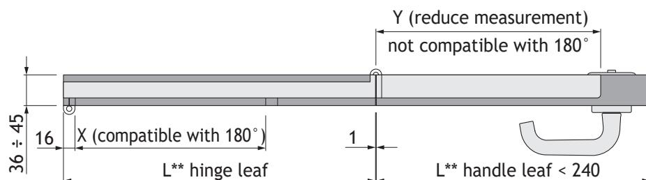
(B): if the handle leaf<sup>(1)</sup> is less than 390 mm wide, Y<sup>(2)</sup> must also be reduced.
