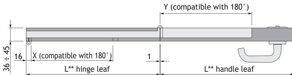
(A): if the handle leaf<sup>(1)</sup> is less than 240 mm wide, Y<sup>(2)</sup> must also be reduced.
