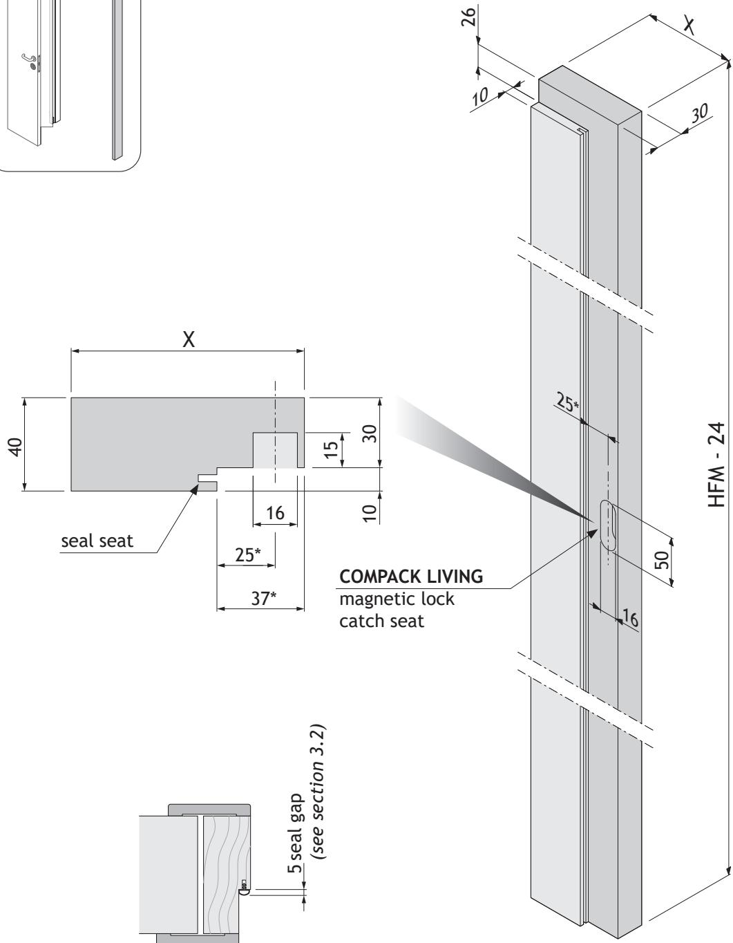
The dimension marked with (\*) vary according to the seal gap dimensions.
